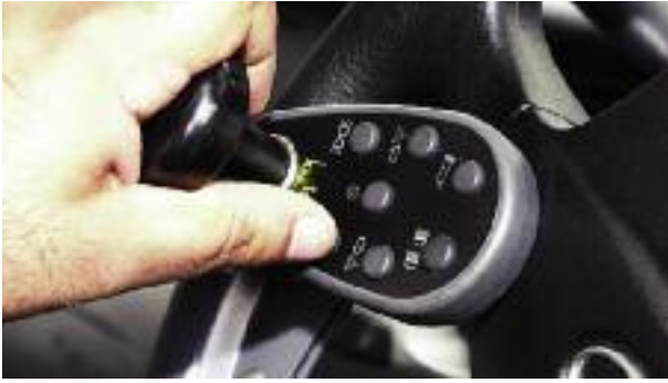
Steering knob combined with wireless secondary controls – Autoadapt
