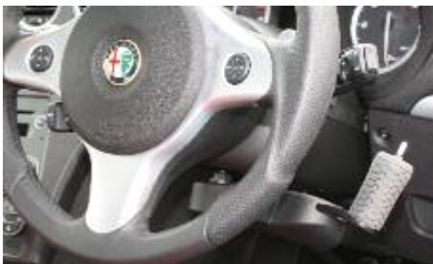
Jeff Gosling single lever accelerator and brake – here fitted with optional indicator switch
